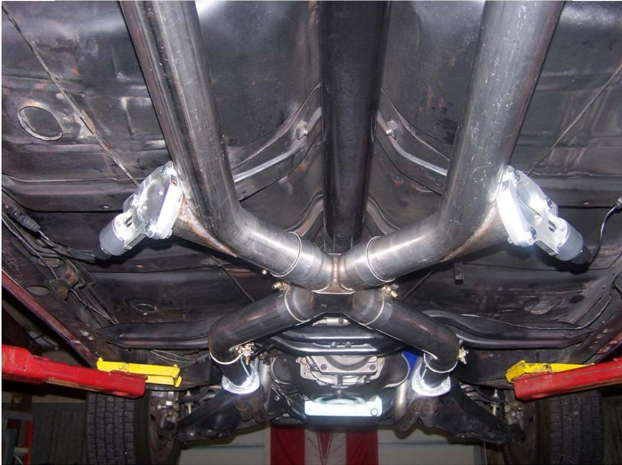
help again. We got all of the pipes, mufflers, hangers and clamps installed and tightened down to what we thought was tight. We fired up the engine and found several leaks. Another call to Pypes and we were told you really need to tightened the clamps down to where the two ends are almost touching. We decided to get some muffler sealer and retighten all the clamps. Once the sealer was installed, all the clamps tightened, everything was sealed and quiet.
